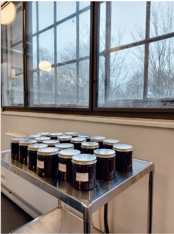
Fig. 3: Selection of microcosms with peat soil from Nydam Mose used to treat archaeological iron samples. © Jacob Frydendahl
