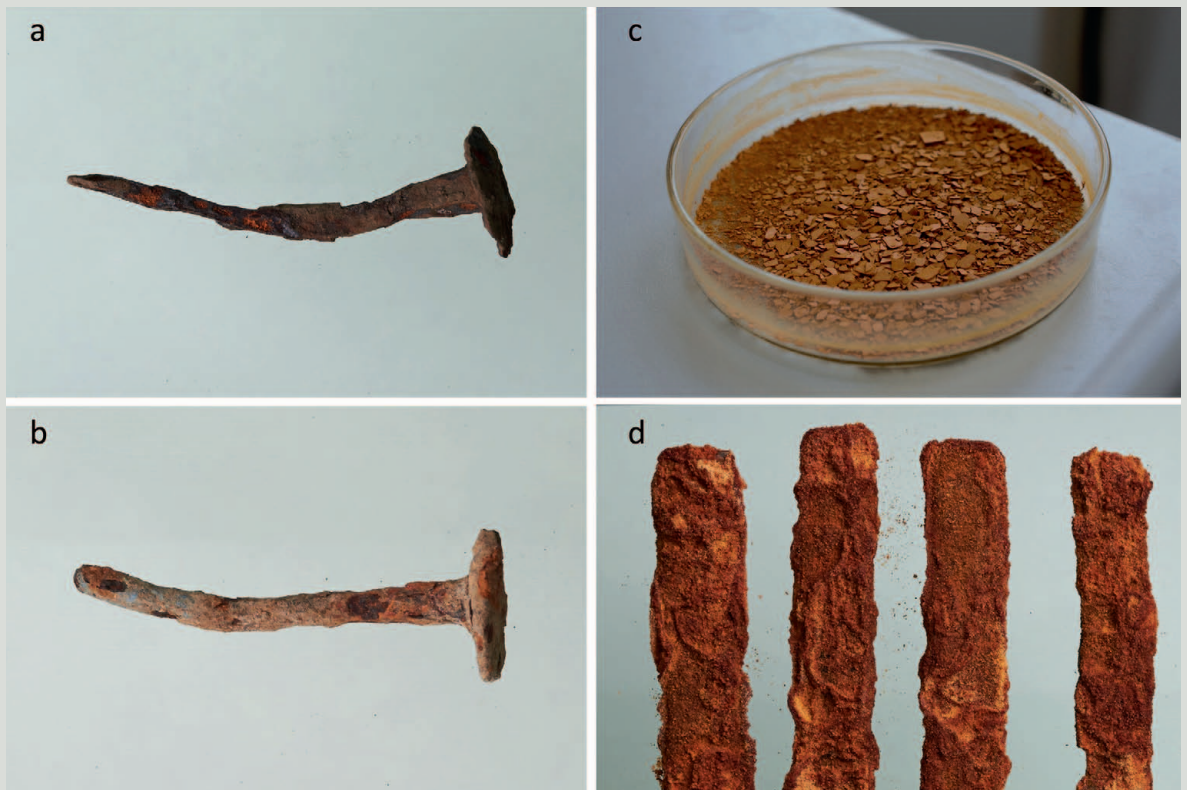
Fig. 4: Examples of sample material. a) iron nail from the rural archaeological site, b) iron nail from the urban archaeological site, c) synthetic akageneite, d) corroded iron coupons. © Jacob Frydendahl
